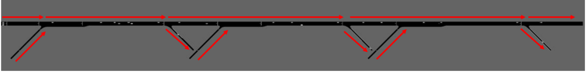
Figure 7.8: This figure illustrates the I-94 domain. The red arrows denote the traffic flow directions. There are four traffic inflows: one highway inflow (leftmost) and three ramp inflows. There are also four traffic outflows: highway outflow (rightmost) and three ramp outflows.
