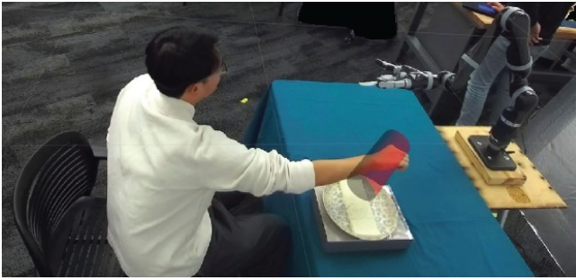
Figure 6: Vision system for detecting and estimating the pose of the human arm in the scene.
